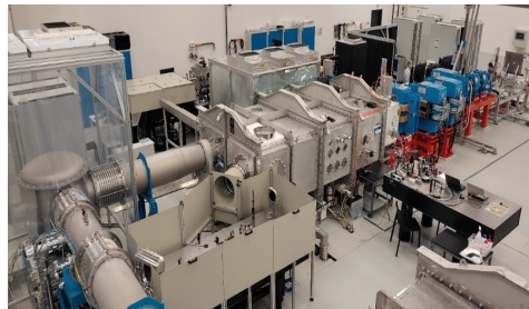
Figure 1: Photo of the ELIMAIA beamline, showing an interaction chamber, ion beam transport (blue and red), and different diagnostic stations.
